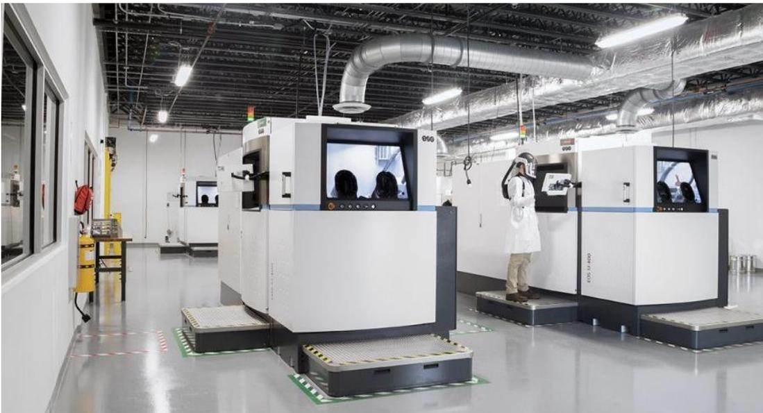
**Figure 6: EOS AM Machines at Sintavia**
