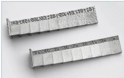
A view of the two test components Sintavia printed in order to show the effects of gas flow within a metal 3D printer. Note the rough surface finish and discoloration of the top piece, which was oriented away from the gas flow inside the build chamber. A side-facing view (above) reveals a rounding and thinning of the upper walls as the print angle increases.
